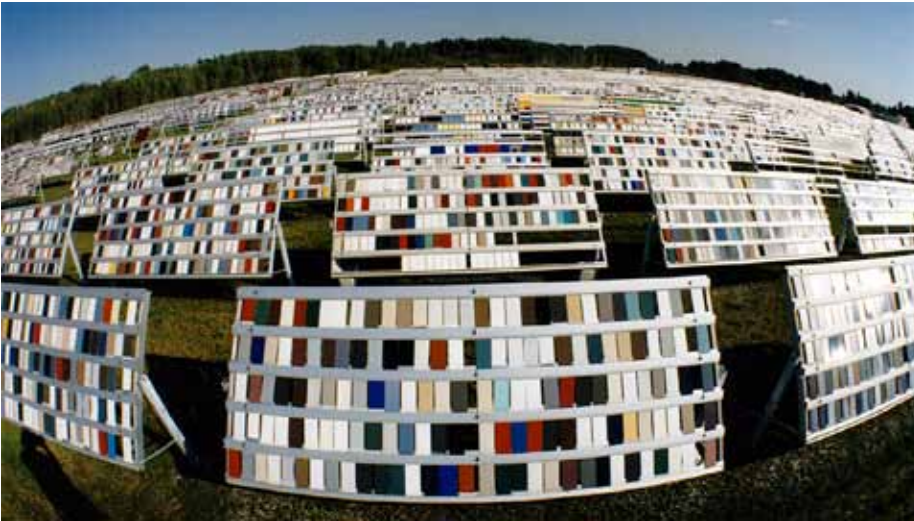
Figure 6 - “Fish-eye” view of static exposure racks in South Florida, a major benchmark location for coatings testing
