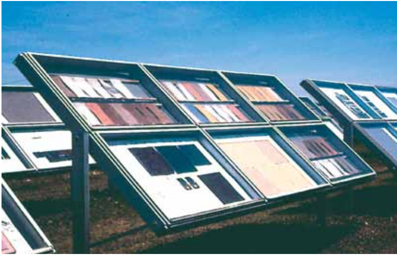
Figure 11 - Exposure behind single strength window glass for testing interior products
