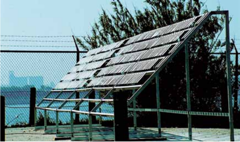
Figure 12 - Coatings on exposure at the North Sea corrosion test center in Hoek Van Holland, The Netherlands
