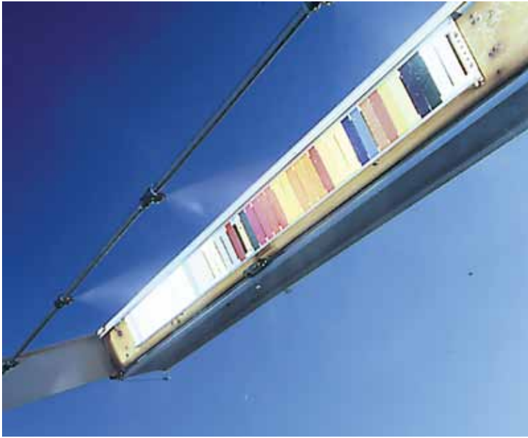
Figure 14 - Target board with water sprays during sun tracking for thermal shock
