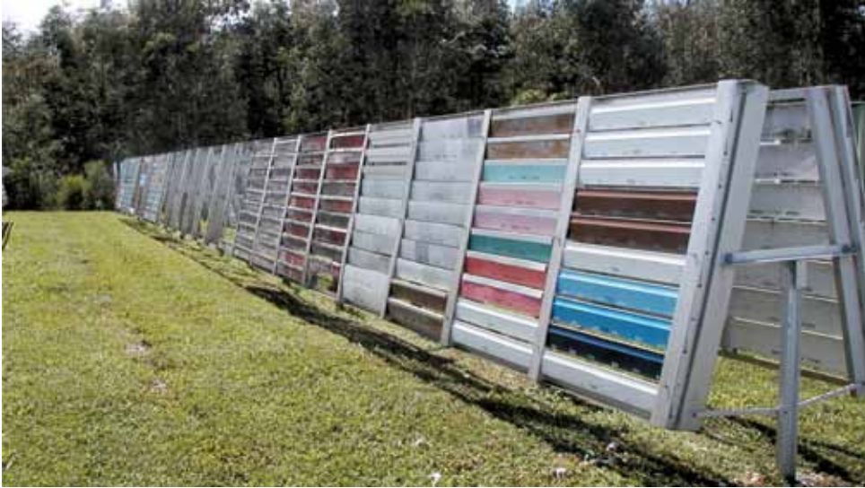
Figure 9 - "Trade panel" test specimens in vertical exposure are offset to avoid cross-contamination by moisture run-off. Paint samples can also face away from the sun for mold and mildew growth studies
