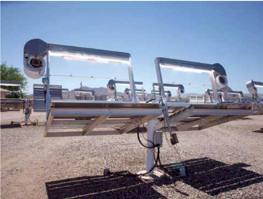
Figure 13 - EMMA/EMMAQUA Fresnel solar concentrator
