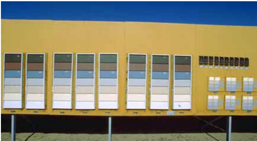
Figure 8 - Test specimens on a 90° vertical exposure rack
