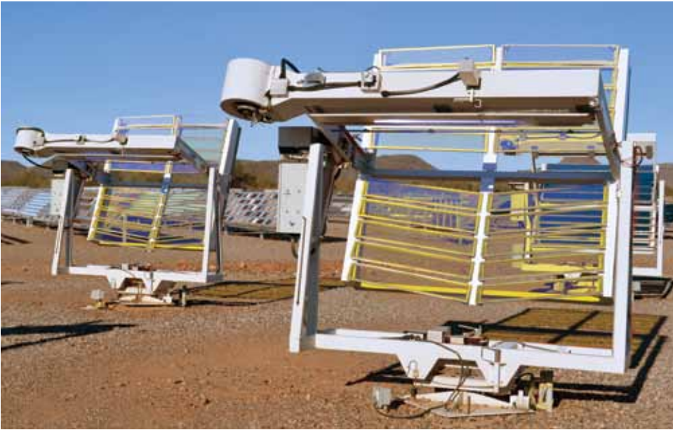
Figure 16 - UA-EMMA/EMMAQUA with “cool mirror” technology
