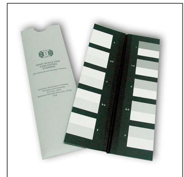
Figure 3. The AATCC and ISO Gray Scale for Staining. Ratings run from 1 to 5 in steps of 0.5 units.
