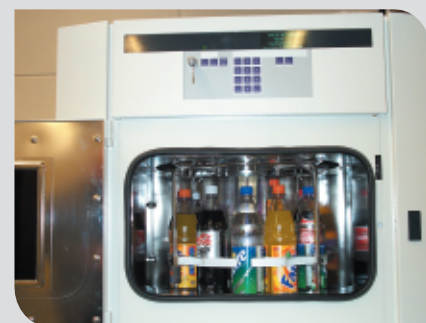
Special sample carousel in a Xenotest Beta+ to hold customary bottles
