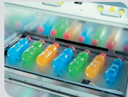
PET bottles in a SUNTEST XXL+ flatbed xenon exposure system
