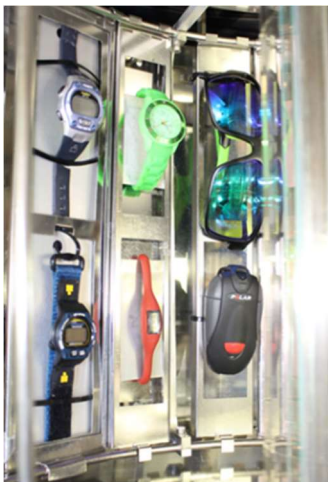
Above: Atlas Ci4400 with sample holders SL-3T and CD-3T. Below: Xenotest Beta+ with sample holders narrow and wide
