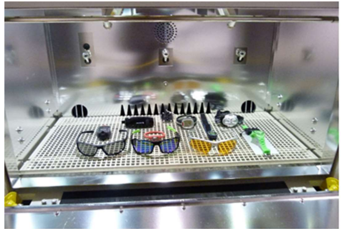
Left: Ci4400 Weather-Ometer® (rot. rack, 7300 cm 2 exposure area. Right: SUNTEST® XXL+ (flatbed, 3000 cm 2 exposure area)
