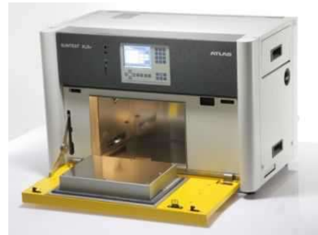
ASLT inside Atlas SUNTEST XLS+ with StoreLight filter, CHT 22 °C: Test Duration: 5 days
