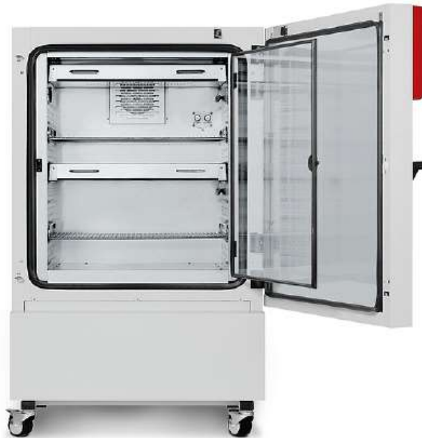
ASLT inside climate chamber with white fluorescent light, CHT 30 °C: Test Duration: 8 Weeks*
