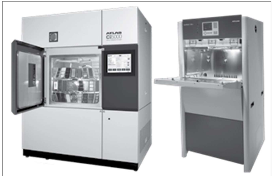
Figure 6: Ci5000 Weather-Ometer® rotating rack xenon instrument and SUNTEST® XXL+ flatbed xenon instrument
