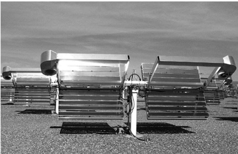
Figure 4: EMMAQUA® solar concentrator for accelerated weather testing.
