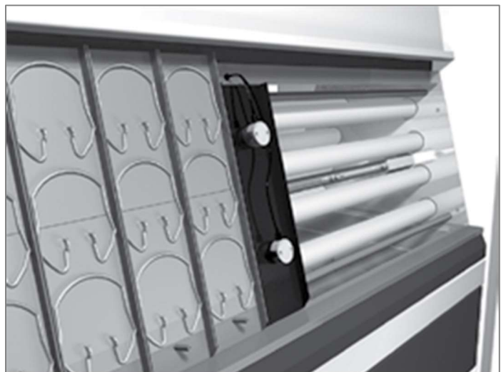
Figure 7: Inside of an Atlas UVTest showing UV lamps, Black Panel Temperature Control and ergonomically designed specimen retention clips.
