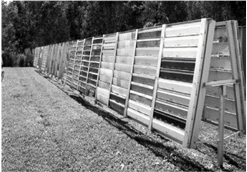
Figure 2: South (shown) and north facing paint panels in Florida. Panels are offset to avoid runoff contamination.
