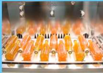
Test conditions for simulation of extended hot summer daylight exposure in SUNTEST XXL+FD
