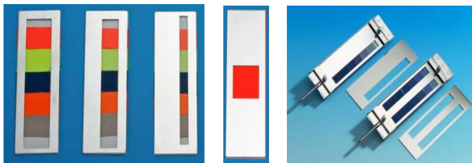
Figure 4 (left to right): ISO 105-B02 Exposure Method 2 cover masks, AATCC cover mask, ISO 105-B02 Exposure Method 3 (Marks & Spencer) cover masks.
