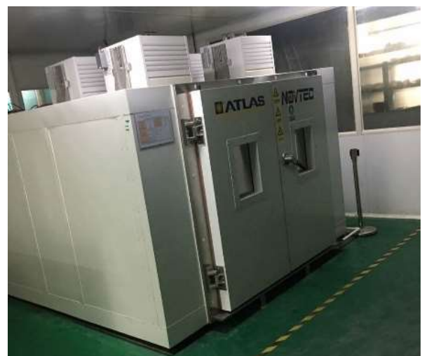
Figure 2: SEC Walk-in chamber with four units of SolarConstant MHG 4000.
