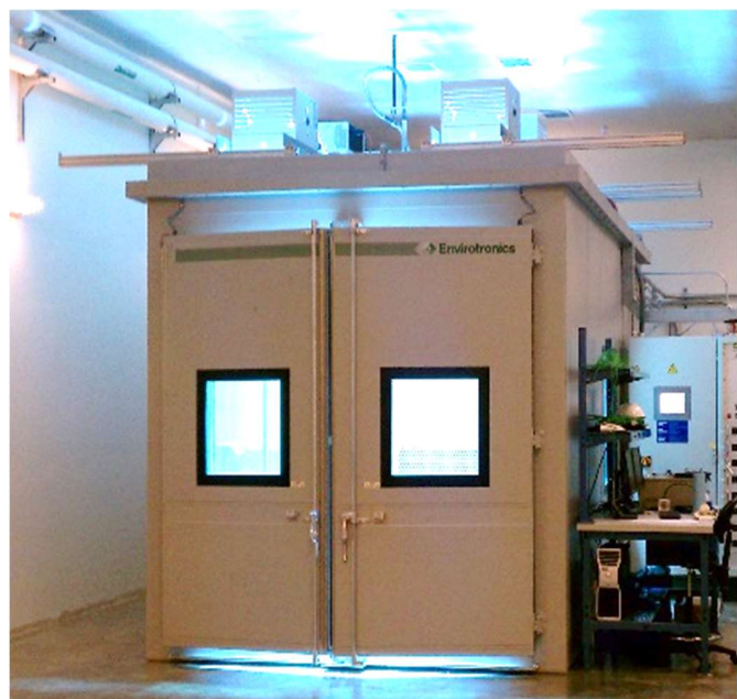
Figure 5: Customized Walk-in MHG solar test chamber using 4x SolarConstant MHG MIL luminaires.
