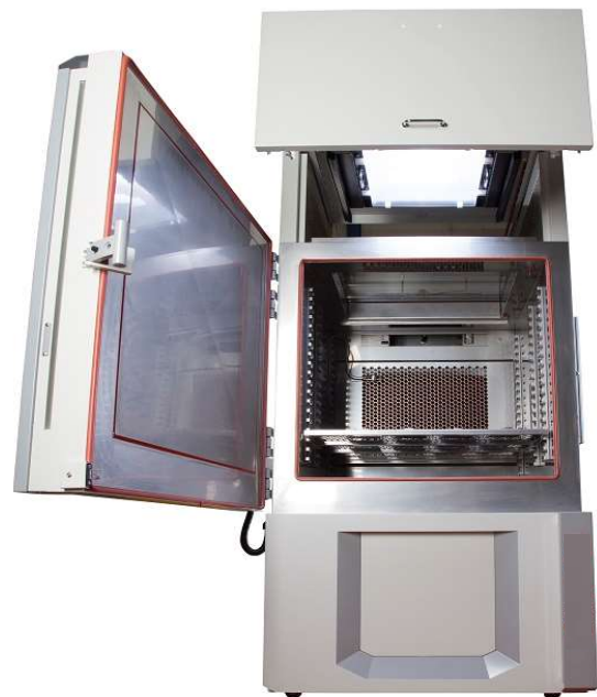
Figure 1: SEC chamber with SolarConstant MHG 4000; size ca. 1000 l.
