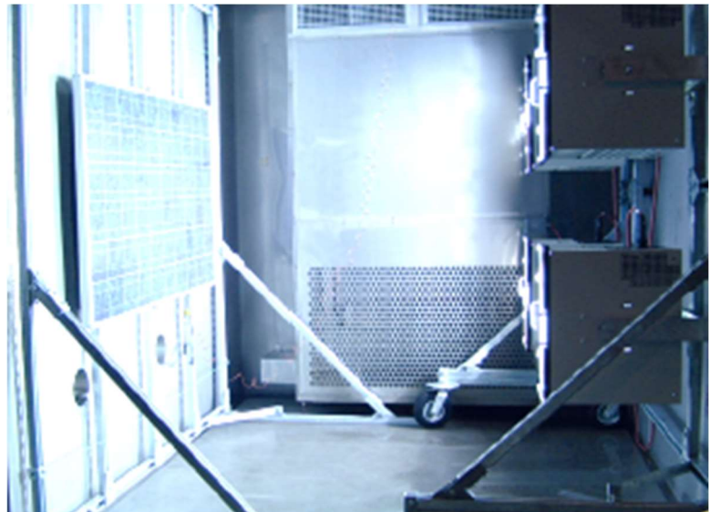
Figure 6: Customized rack with MHG solar simulator using 4 SolarConstant MHG luminaires.
