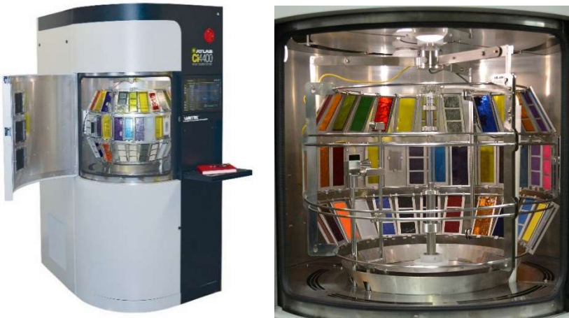
Figure 1. Atlas Ci4400 Weather-Ometer® xenon-arc instrument with a rotating rack configuration
