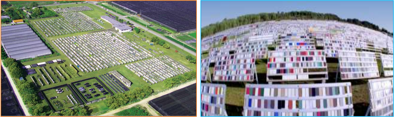
Figure 5. Outdoor exposures in a sub-tropical climate of South Florida, representing one of the ‘benchmark’ climates for automotive exterior weathering testing.
