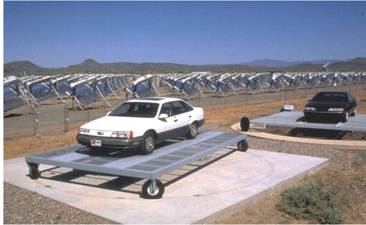
Figure 4. Sun-tracking carousel to measure automotive interior surface temperatures. By tracking the sun and orienting the vehicle at different angles with respect to the sun, maximum surface temperatures can be measured on all surfaces
