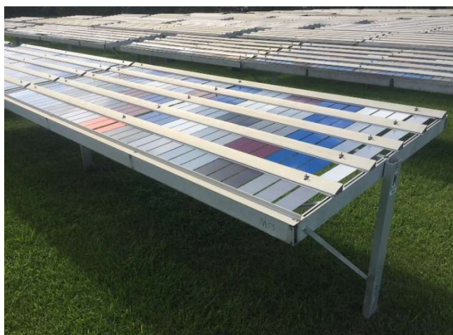
Figure 9: Standard 5° exposure racks at benchmark exposure site near Miami (Florida)
