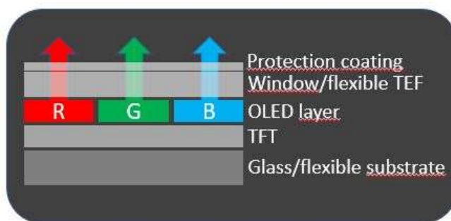
Schematic OLED display structure
