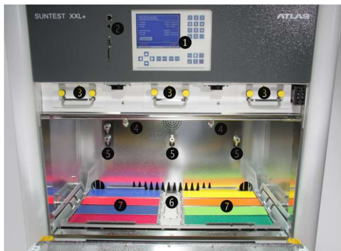
Atlas SUNTEST XXL+: (1) Touch screen user interface, (2) Ethernet, USB, SD Card, RS232, (3) Light Cassette incl. xenon lamp, optical filter, (4) Water spray nozzles, (5) Light monitors, (6) Black Panel Temperature sensor, (7) Specimens
