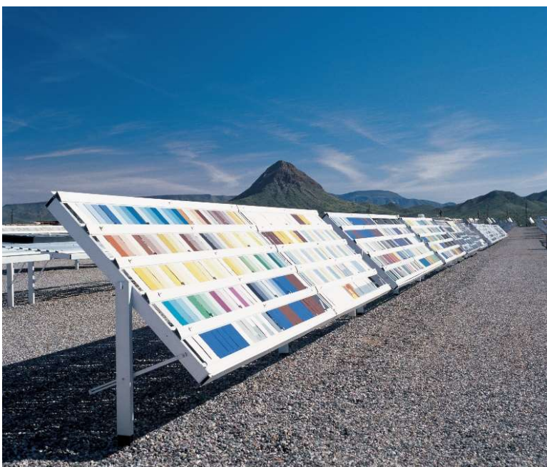
Figure 4. Exposure Rack in Phoenix/Arizona, 45° facing south
