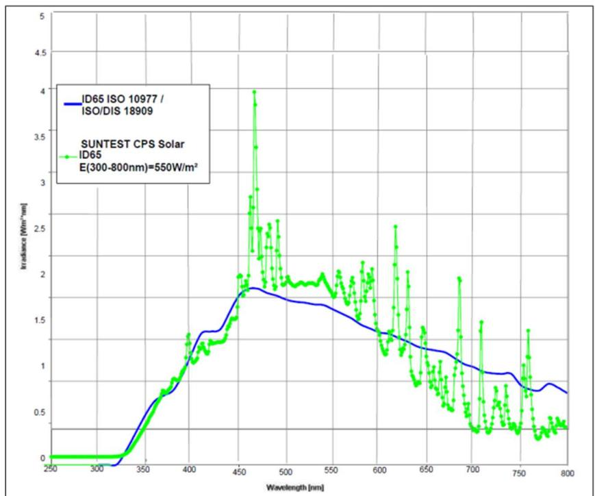
**Figure 1:** Spectrum Comparison between ID65 (ISO 10977 / ISO DIS 18909) and SUNTEST CPS+ with Solar ID65 filter system.
