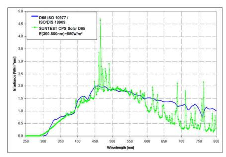
Figure 2: Spectrum Comparison between D65 Daylight (ISO 10977 / ISO DIS 18909) and SUNTEST CPS+ with Daylight filter system.
