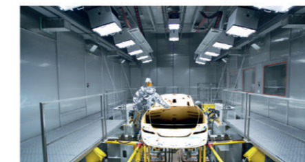
Climatic chamber with 4-poster / dynamic road simulation with solar simulation
