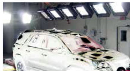
Climate test chambers with dynamometer and solar simulation
