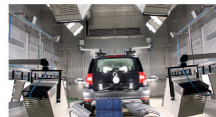
Solar Heat Load test chambers (Day Cycling)
