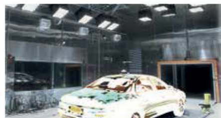
Climate test chambers with wind tunnel and solar simulation
